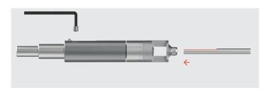
When inserting the drill bit, make sure that the planar surface of the drill bit points in the direction of the pin
